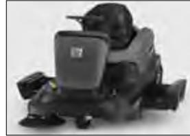
The two drawer-type sweeping containers have large joint capacity of 13 gallons and are easy to empty even when filled to capacity
