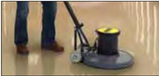
Kärcher floor machines and burnishers provide power and versatility for buffing, polishing, scrubbing and stripping.
