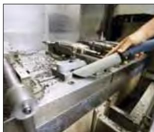
Chippings and shavings kit, e.g. for cleaning metal- or wood-processing machines.
