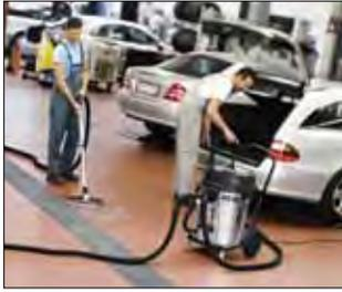
The Y-piece kit makes it possible to connect two suction hoses to one machine. This makes it possible to clean multiple areas at the same time.
