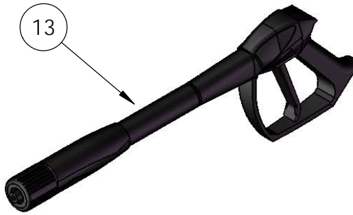
GUN, 3700PSI, 8 GPM, M22 IN, M22(F) OUT (PART NO. 7103518)
